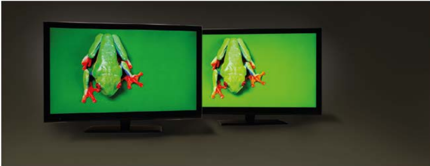
Figure 1 | Comparison between a liquid-crystal display television screen using a Quantum Dot Enhancement Film (left) and a standard one (right). Photo courtesy of Nanosys/Thom Sanborn.
