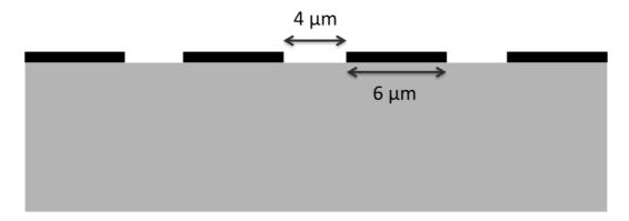
Using an anisotropic etch where the etch rate in z is 3 times the etch rate in x,
