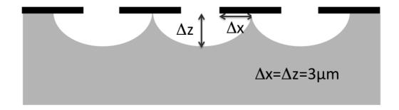
**Exercise 4: Anisotropic etch:** etches at a different rate in z and x. Consider the following substrate (gray) with an etch mask (black).
