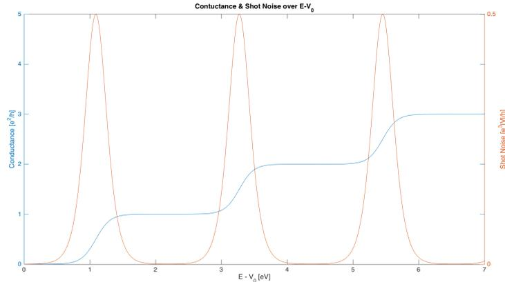
**Figure 6:** Conductance and Shot noise, superimposed as a function of  $E - V_0$ . Note that these calculations are only valid for small  $|V|$  and in this situation it is simply a scaling factor.
