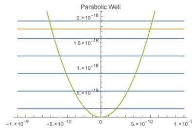
**Figure 5:** Cross section of potential in  $x$  direction at  $y=0$  (i.e.  $\omega_y$  controlled part) with yellow line being  $E - V_0$ , and the blue lines being the quantised energies of the quantum harmonic oscillator
