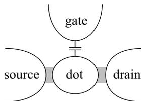
Figure 1: Structure of a SET. The current through the island can be controlled via the gate terminal.
